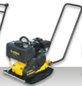
BVP 12/50 A Operating weight: 72 kg Centrifugal force: 10 kN Working width: 300 mm
