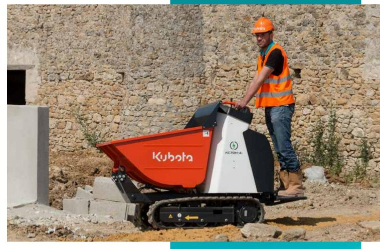
Battery (V / Ah): 48 / 120 Machine weight (kg): KC70H-4e : 645 KC70VSL-4e : 740 Payload (kg): **700**
