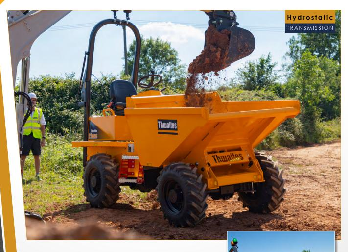
The Thwaites 2 Tonne Front Tip, Stage V dumper is manufactured with contractors and hirers in mind – ensuring operator safety, reducing risk on site and improving performance. Powered by an 18.4 kW 3-cylinder Yanmar engine, delivering 107 Nm max torque for optimum traction and control. The Thwaites 2 Tonne Front Tip is also available with a Manual Transmission.
