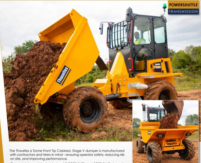
The cab is impact tested to level 2 ROPS 3471 and FOPS 3449. As such all Thwaites cabbed dumpers are approved for use by the UK Major Contractors Group. Front Tip dumpers allow the machine to be easily and safely unloaded, with a straightforward tipping action that places the full bucket of spoil exactly where it is required.
