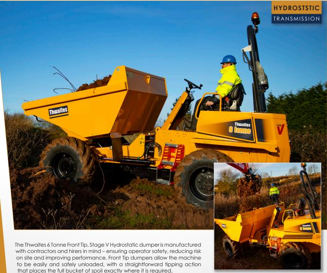
Powered by a 3.3L Yanmar turbo diesel engine fitted with a DPF to comply with EU stage V emission regulations, you benefit from 53.7 kW peak power, 295 Nm of torque and no AdBlue requirement.
